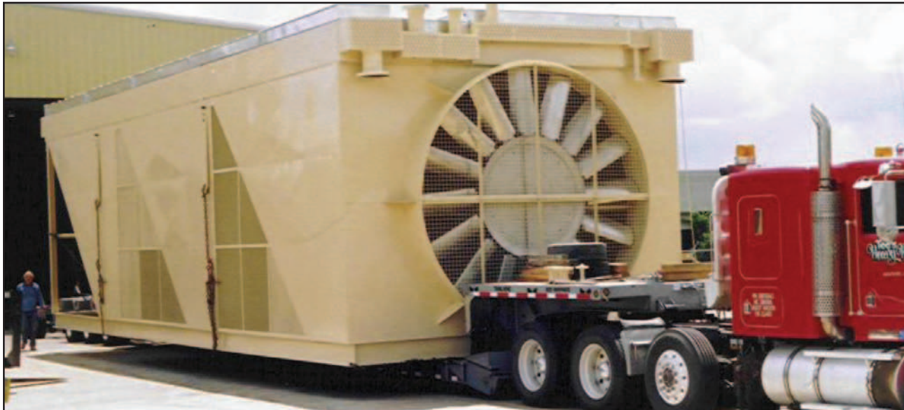
■ Shown here at ACE's shop in Broken Arrow, Oklahoma, what will be used on a PAMCO-Stewart and Stevenson-built compressor package by Public Service Company of Colorado. The cooler measures 53 ft. long, 18.5 ft. wide and 16.5 ft. tall (16.15 m x 5.64 m x 5.03 m) and weighs approximately 110,000 lb. (49,900 kg)
